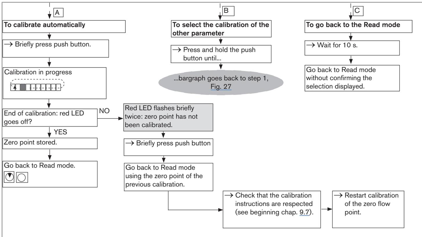
Fig. 28 : Calibration of the zero flow point, part 2
