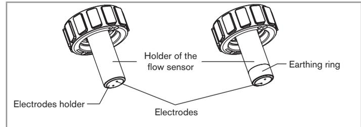
Fig. 3 : Parts of the flow sensor holder in stainless steel (left) or in PVDF (right), devices with a G2" nut
