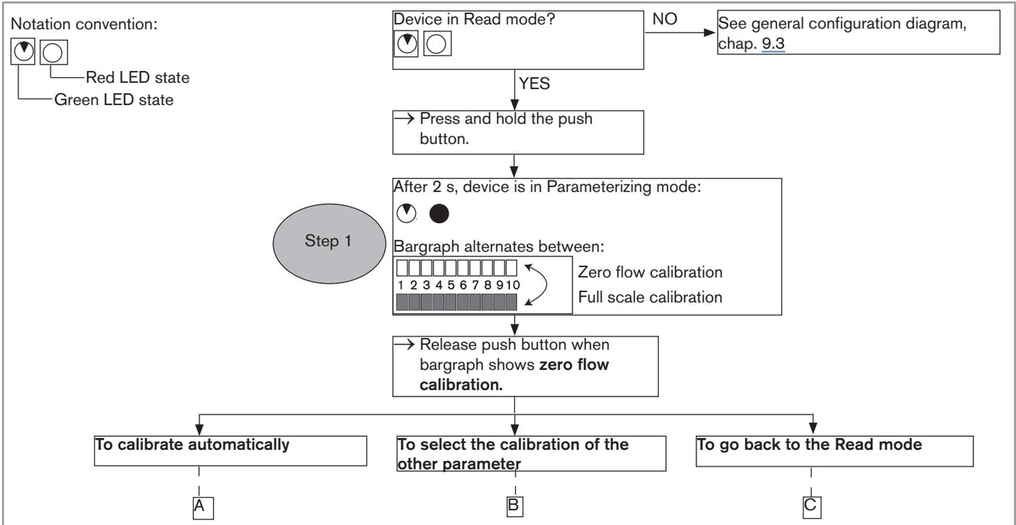
Fig. 27 : Calibration of the zero flow point, part 1
