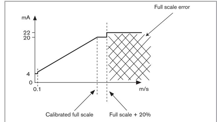
Fig. 30 : Relation between the measured fluid velocity and the value of the current output
