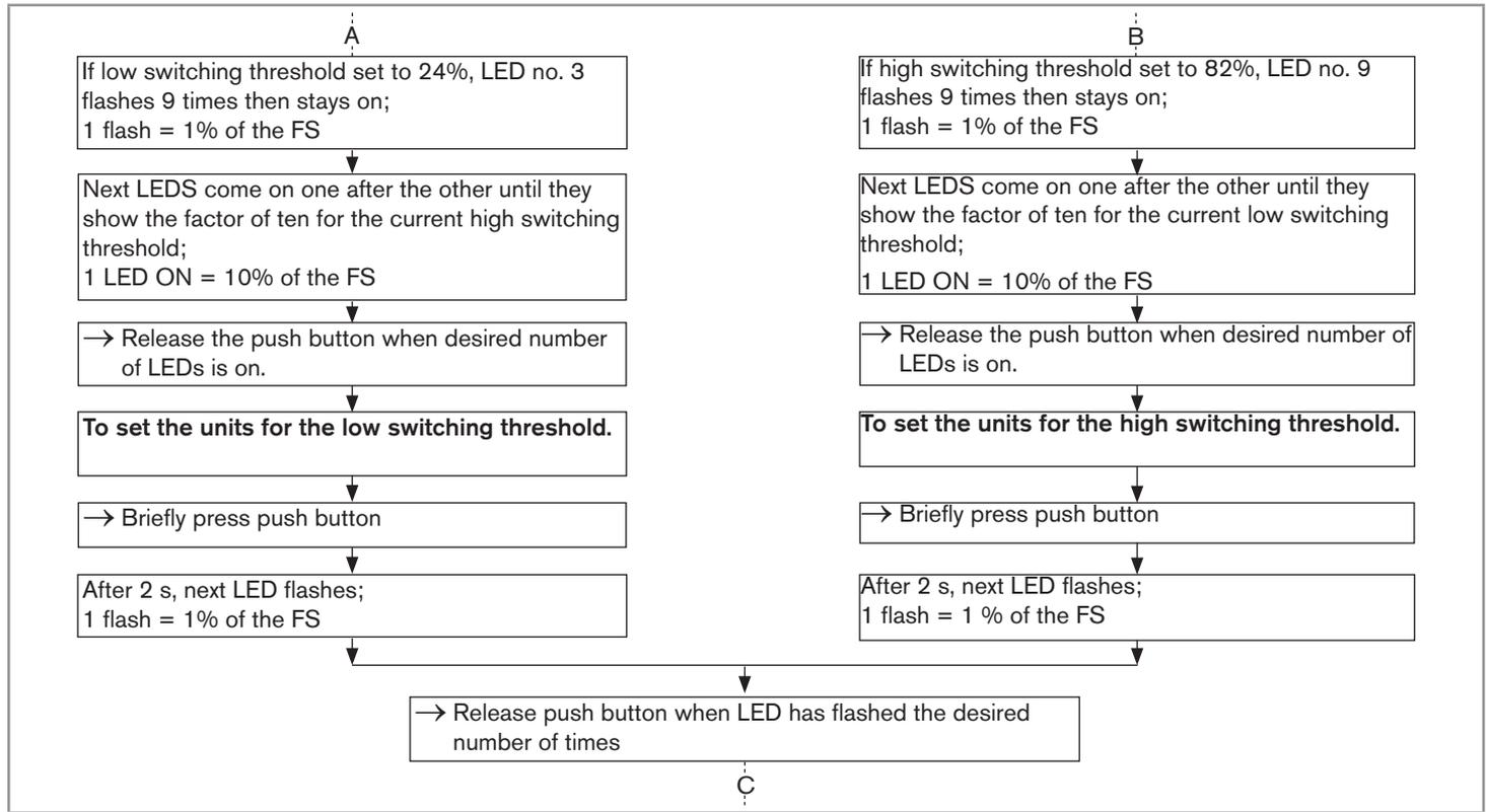
Fig. 41 : Setting the relay switching thresholds, part 2
