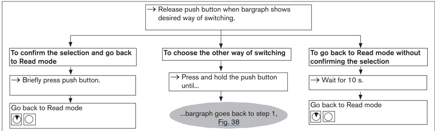
Fig. 39 : Choosing the relay switching way, part 2
