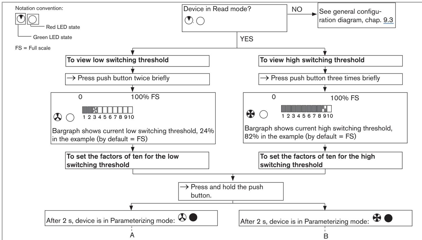
Fig. 40 : Setting the relay switching thresholds, part 1
