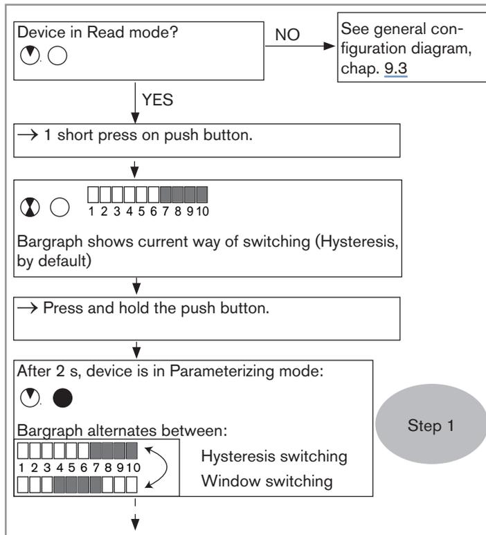
Fig. 38 : Choosing the relay switching way, part 1
