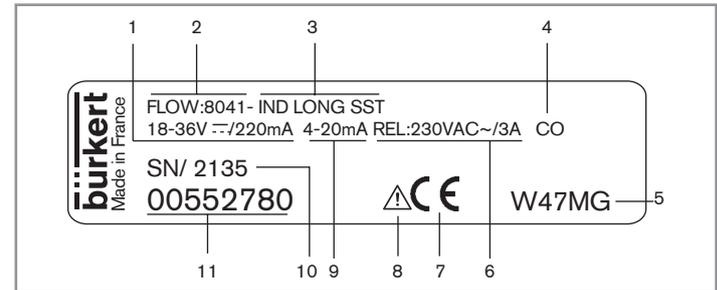
Fig. 2 : Name plate of the device (example)
