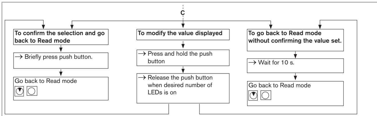
Fig. 42 : Setting the relay switching thresholds, part 3
