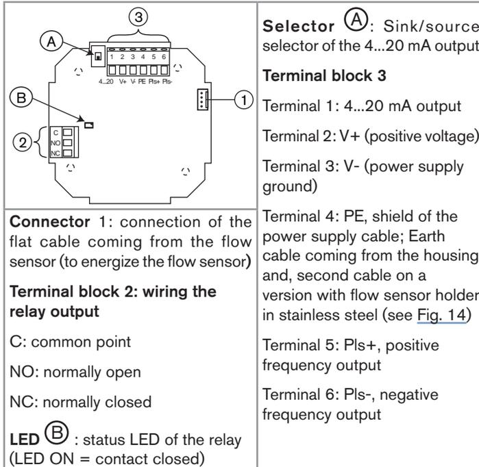
Fig. 13 : Terminal assignment
